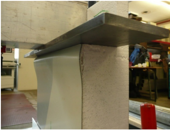
Fig. 3.5: Crippling of the load application area
