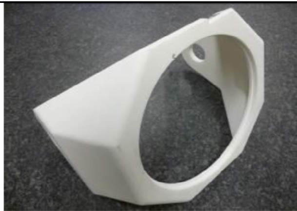
Part with warpage, weight: 657 grams, (original carbon fibre laminated version with a honeycomb core: 170 grams)
