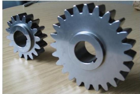
Fig. 3.6-3: Geometry of the FZG test gear Type C.
