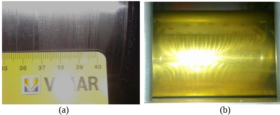
Fig. 3.6-5: Rolling mill (a) and damaged roller (b)
