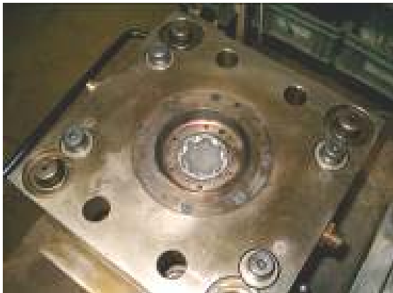
Injection mould after production of 10000 pieces
