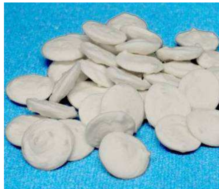
Figure 6 - ReBioFoam starch-based pellets
