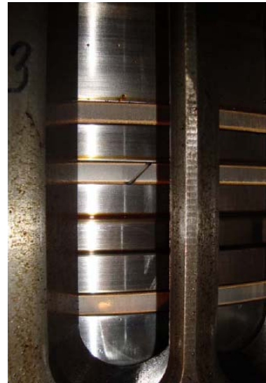
Figure 7.2a (ii) The old guide shoe (top) and the updated low friction version (bottom), and the new three piston ring pack installed on piston (right)
