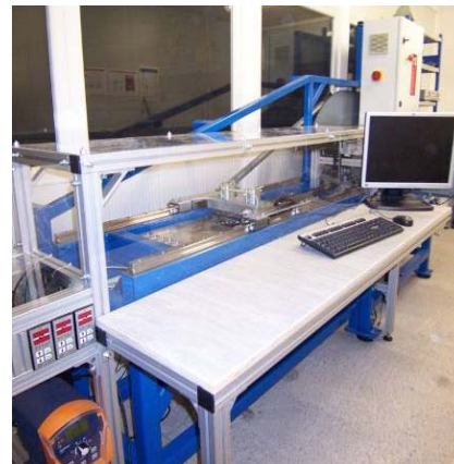
Figure 7.2b(i) The CAD model of the rig and the actual lube oil distribution test rig
