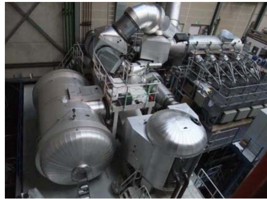
Figure 3.1a. Installation of 2-stage turbocharging system on the 4-stroke (left) and 2-stroke (right)
