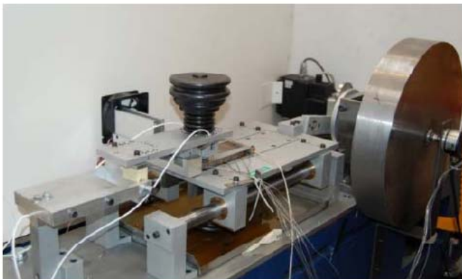
Figure 7.2a (i) The Reciprocating Test Rig (left) and the L16/24 test rig with a new liner mounted (right)
