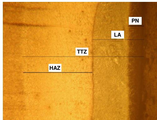
Figure 1-7: Micrograph of a combined treated surface
