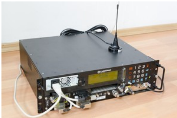
Figure 21 - Independent Digital Repeater (IDR) from Cassidian
