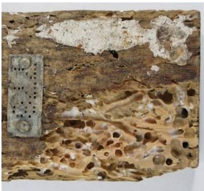
Figure 2. Heavy attack by Teredo navalis . The mollusc penetrates and digests the wood material forming up to one centimetre wide tunnels.
