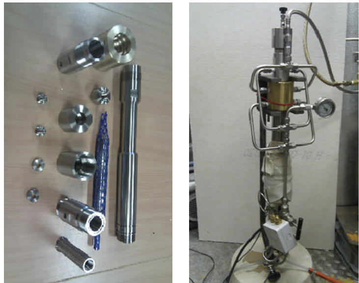
Figure 30: ECT engine parts (left) and assembled engine (right).
