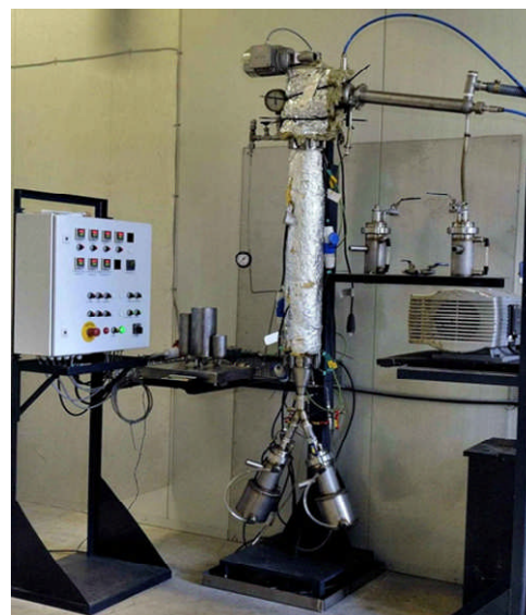
Figure 6: Lab-scale film evaporator to remove water from fast pyrolysis oil
