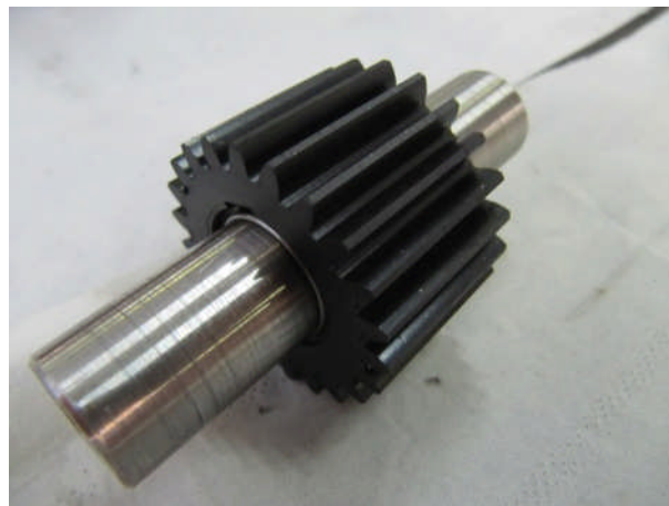
Figure 16: PEEK gear and shaft. Both elements withstood contact with fast pyrolysis oil perfectly.
