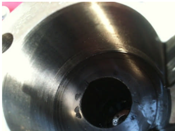
Figure 15: Damages on the graphite buckles on the left side of the NAX10 pump.
