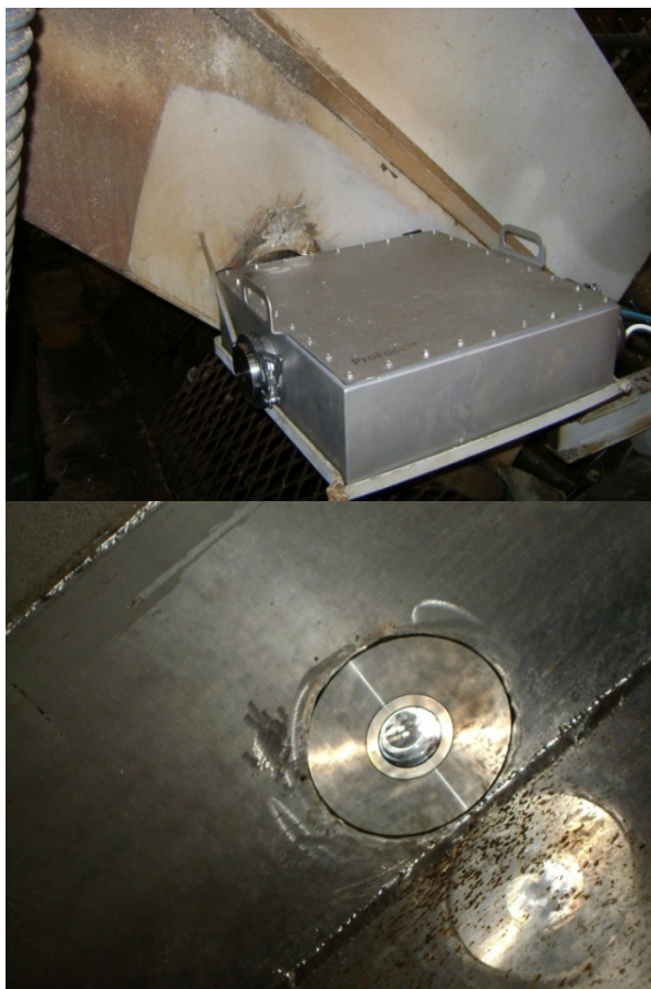
Figure: Integration of the ProFOSS system with the bagasse chute in the sugar mill.
