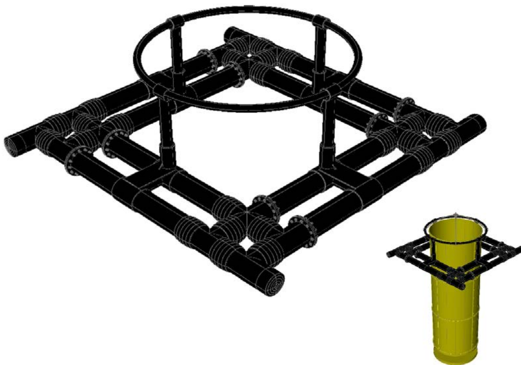
Figure 4. 3-D view of an individual LAMP structure. The insert shows 3-D view of the structure with a mesocosm bag.
