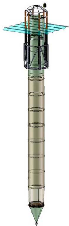
Figure 2. Sketch of a KOSMOS single mesocosm unit.
