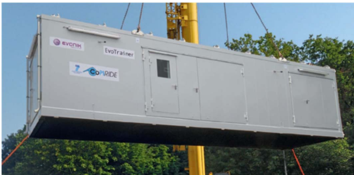
Fig. 6: The mobile EvoTrainer 3G: Infrastructure for product development from lab to production (Source: Evonik).
