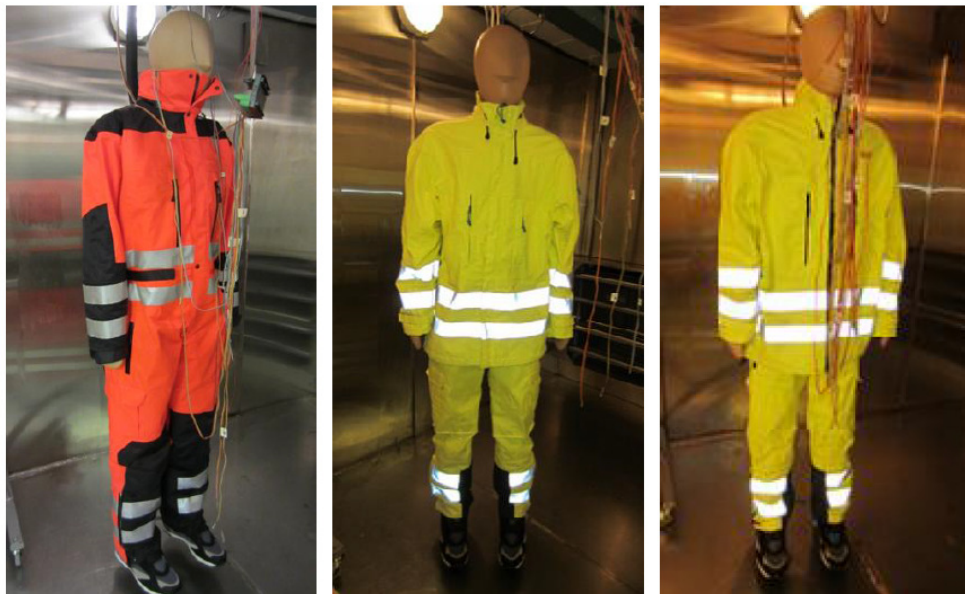
The three prototypes dressed on the sweating thermal manikin
