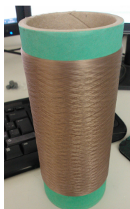
Photocatalytic yarn based on SPEEK/polyolefin blend and its characteristics
