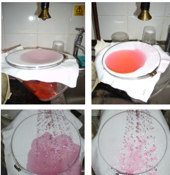
Shower-proof test on untreated cotton (left) and sol-gel treated cotton (right)
