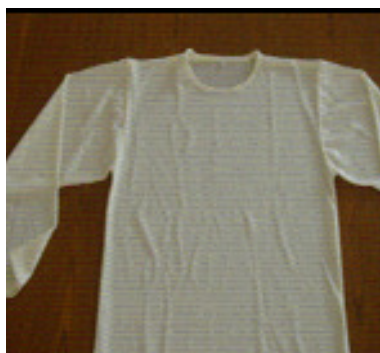
Thermoregulating T-shirt made of bi-component yarns incorporating PCMs that melt at 32 °C
