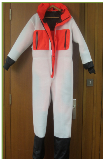
Picture of prototype 1 (inside out) showing the 3D knitted liner providing thermal insulation
