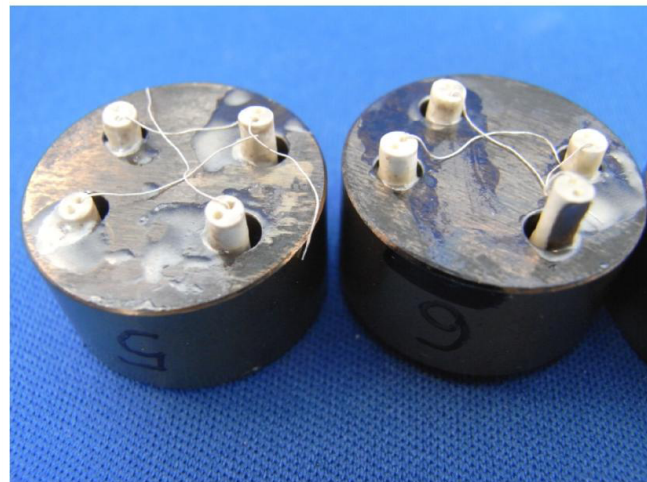
Fig. Pera-3 – Sensor with ceramic tube insulating the wires
