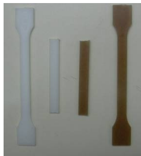
Figure 8: Tensile, flexural and impact standardized test specimens
