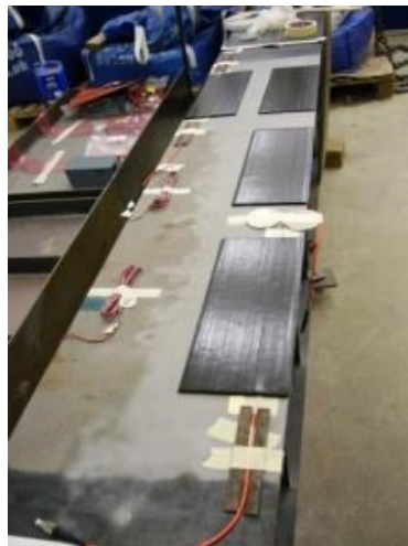
Patch lamination at the bottom flange of a civil engineering application girder
