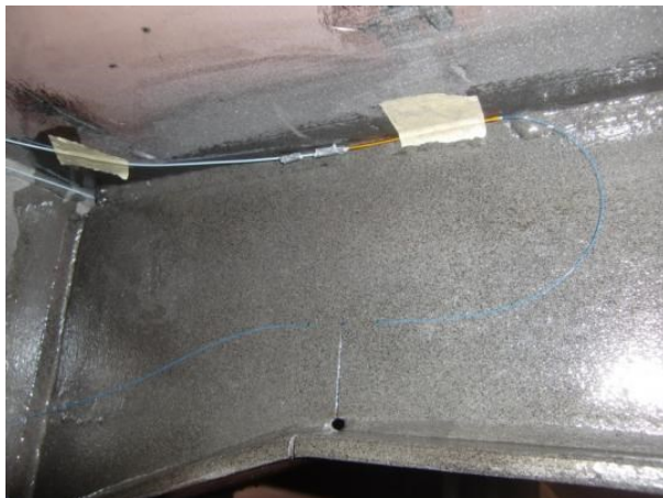
Different types of cracks on the transverse beams of the Catamaran
