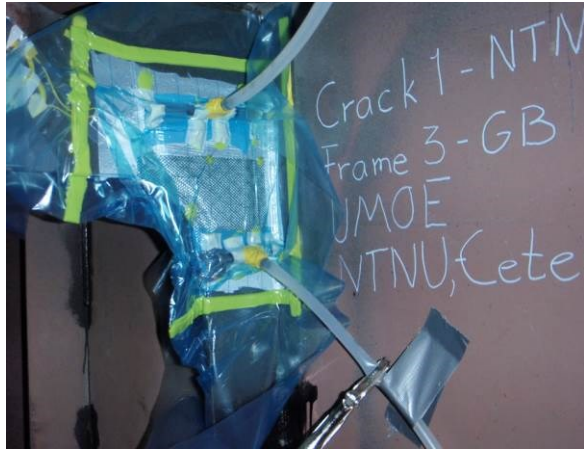
Vacuum infusion of patch repair inside the Catamaran (left) and finished patch (right)
