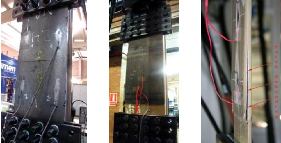
Back side (left) and patched side (middle) of a plate tensile test; patch debonding on a plate specimen (right)
