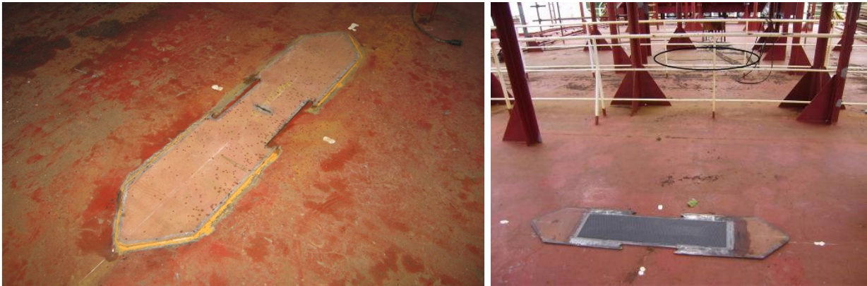
Patch installed on deck of M/V FRANKOPAN – unpatched plate (left), patched plate (right)
