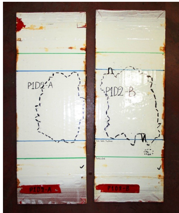
Findings in patched plate specimens after inspection with BONDMASTER device prior to testing
