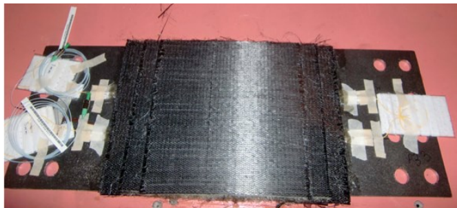
Patched plate test specimens with Optical Backscatter Reflectometry fibres and measurement unit
