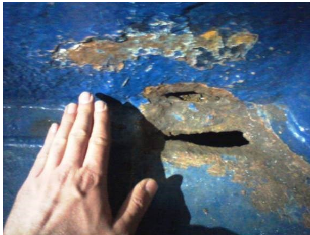
Ro-PAX garage floor repairs – before repair (left), after patch repair (right)
