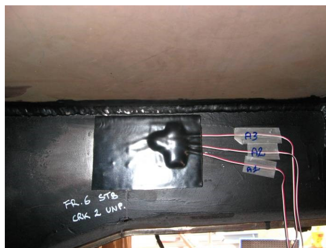
Sensors' wiring at the defects area for monitoring structural response
