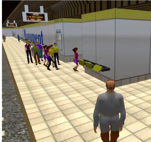
Figure 6: Simulation controlled traveller Avatars following DSS issued evacuation plans (from live trial at Monument metro station)
