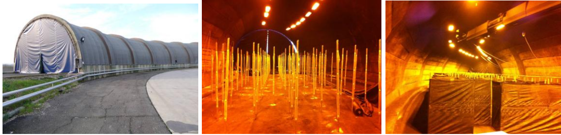
Figure 3: External view of the Montelibretti tunnel, the poles that served as the main structural element of the labyrinth (middle photo) and the labyrinth completely mounted (right photo)
