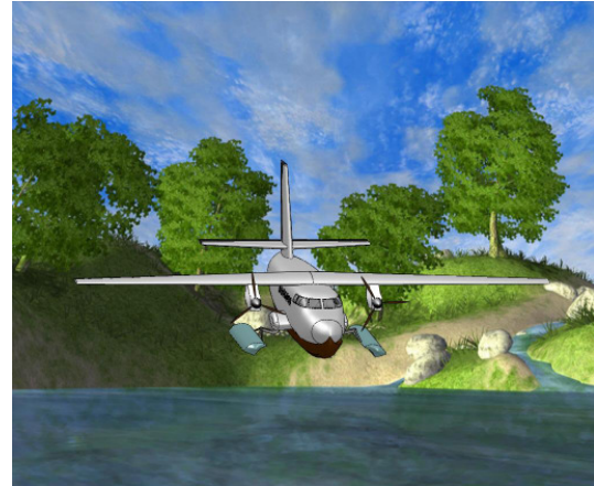
Figure 3-12: Design with retractable floats
