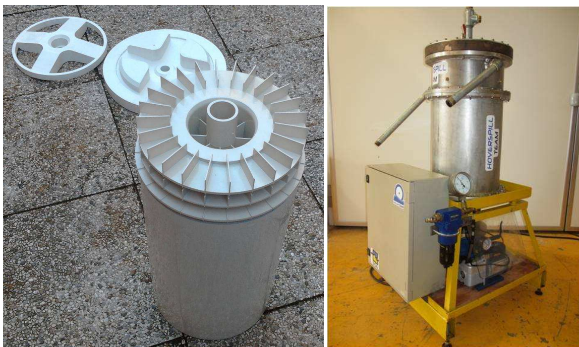
Figure 4: manufacturing of the Turbylec separator prototype. Left: rotor – Right: complete system
