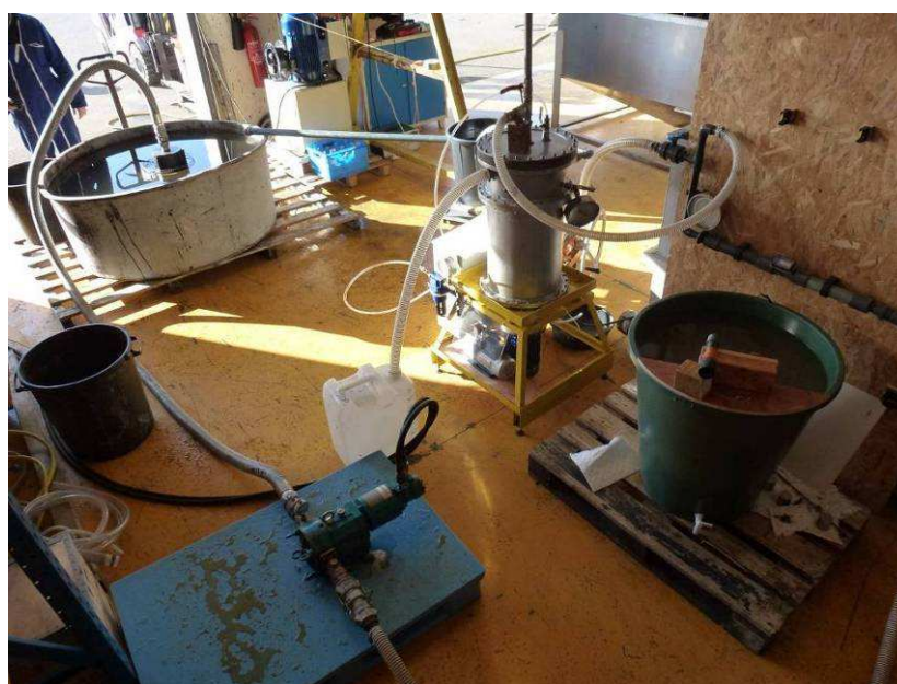
Figure 6: Experimental configuration: skimmer + pump + TURBYLEC.
