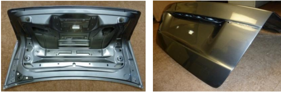
Figure 40 Standard pressed steel part, inner (left), and outer rear surface (right).
