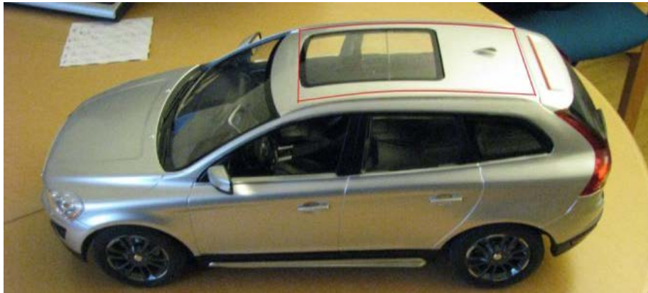
Figure 37 RC car with marked roof area to be replaced by a multifunctional laminate
