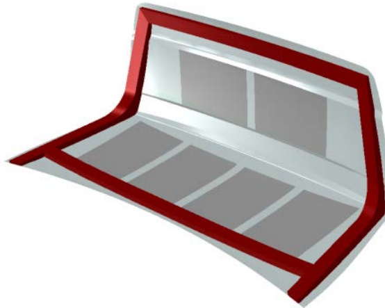
Figure 41 CFRP skin with six MF slabs (grey) and Omega stiffeners (red) laid up over foam core.
