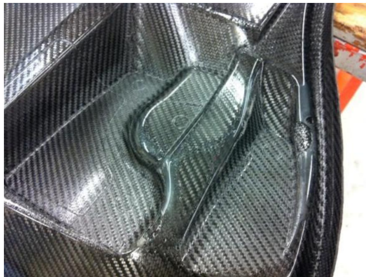
Figure 45 Resin pockets and airbubbles at the radius of the first plenum cover
