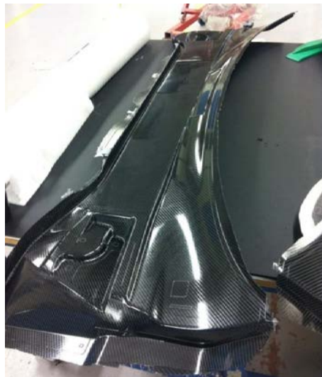
Figure 47 Third and final version of the plenum cover
