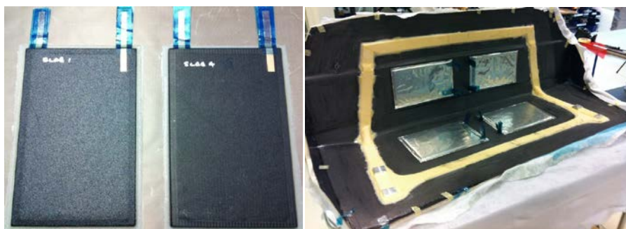
Figure 35 Multifunctional slabs glued to the outer skin.
