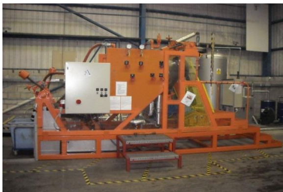
Autoclave used for food waste preparation
