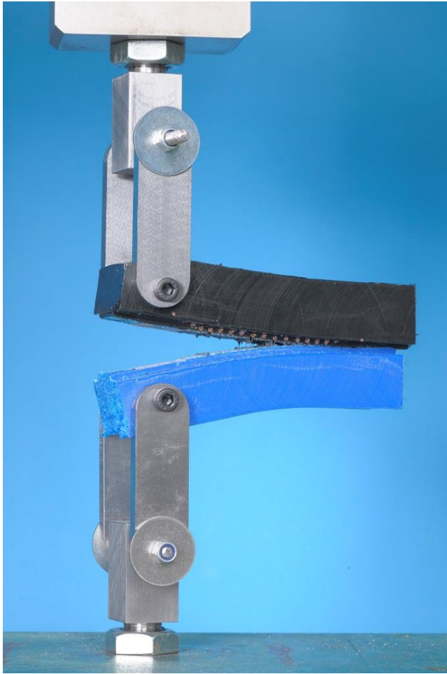
Figure 69 Peel decohesion test.
