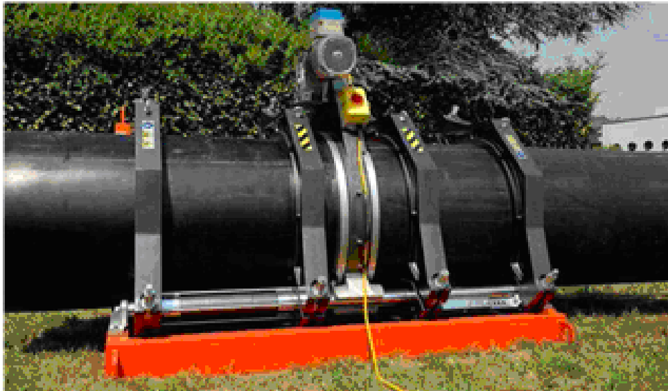
Figure 31 Butt fusion welding of PE pipes.
