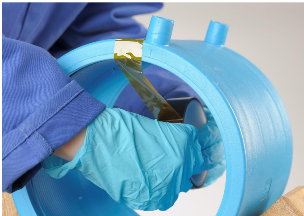
Figure 14 Application of polyimide tape to an EF coupler.
