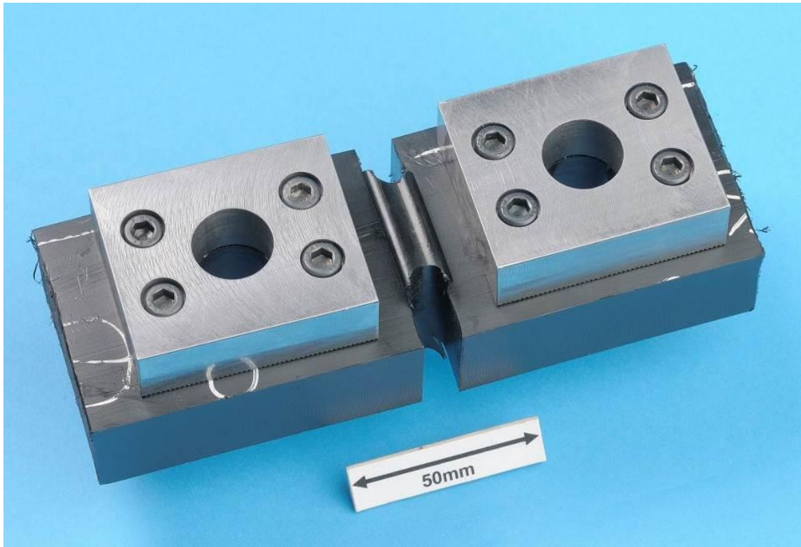
Figure 63 Waisted tensile test specimen with side plates attached.
