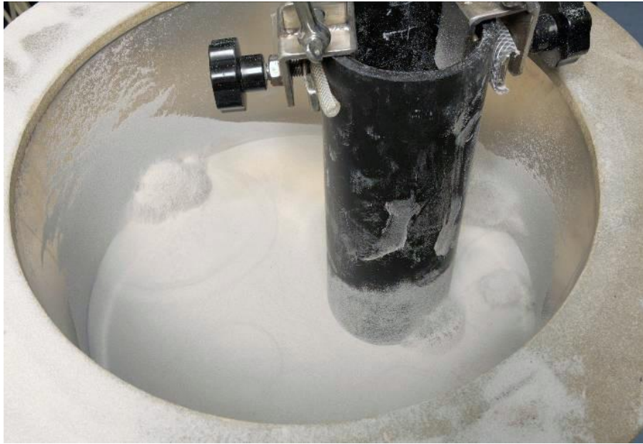
Figure 15 Applying sand contamination to the pipe end using a fluidised bed.
