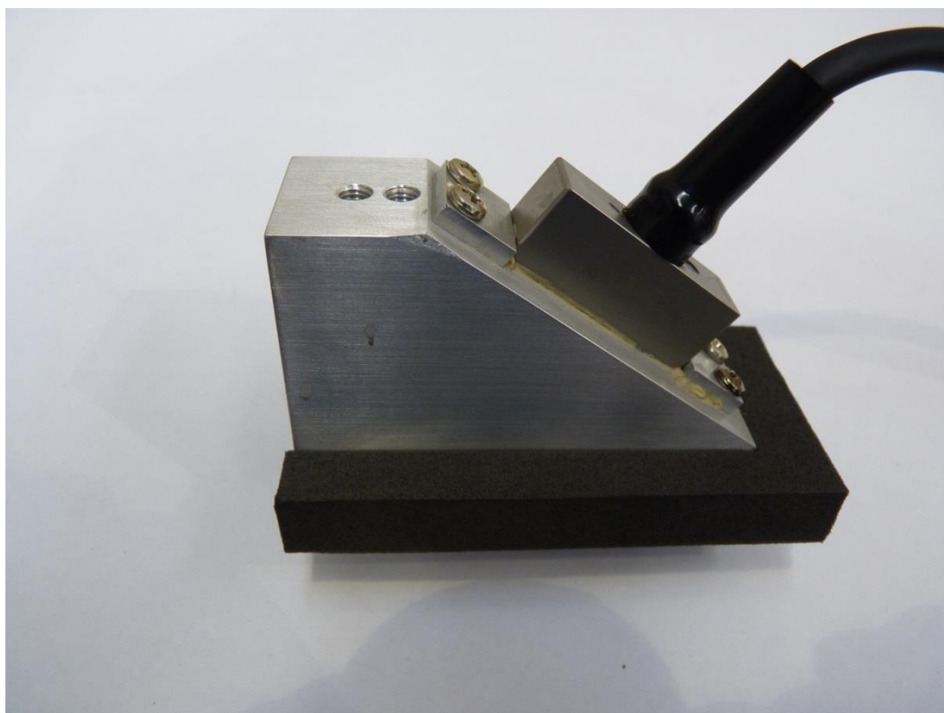
Figure 37 Angled water wedge for inspecting butt fusion joints, with phased array probe and sealing skirt attached.
