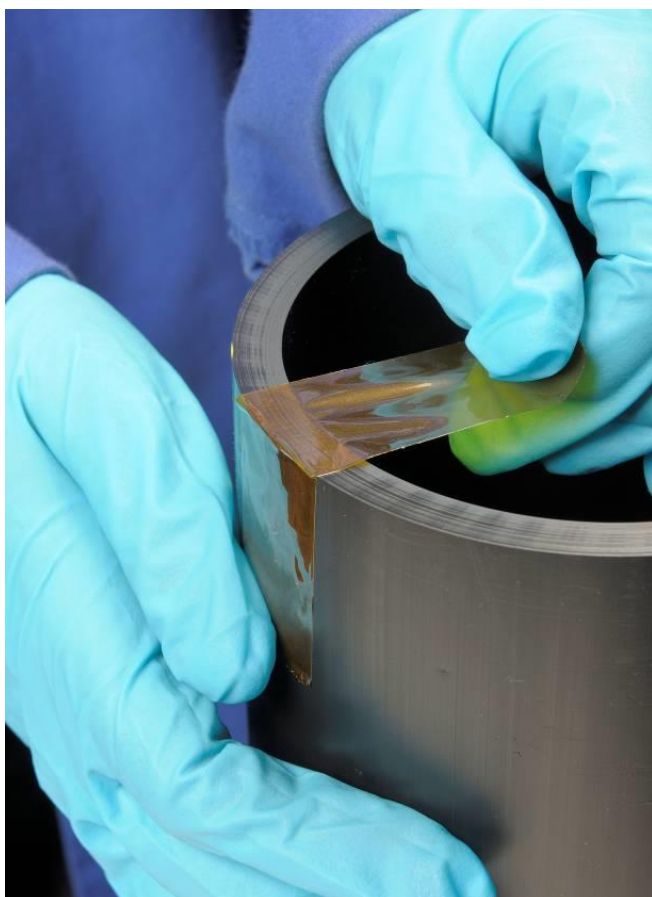
Figure 13 Application of polyimide tape to the trimmed end of a PE pipe.
