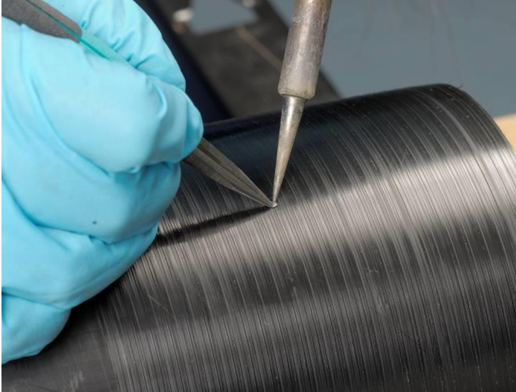
Figure 20 Heat staking aluminium disc to the scraped surface of a pipe for EF welding.
