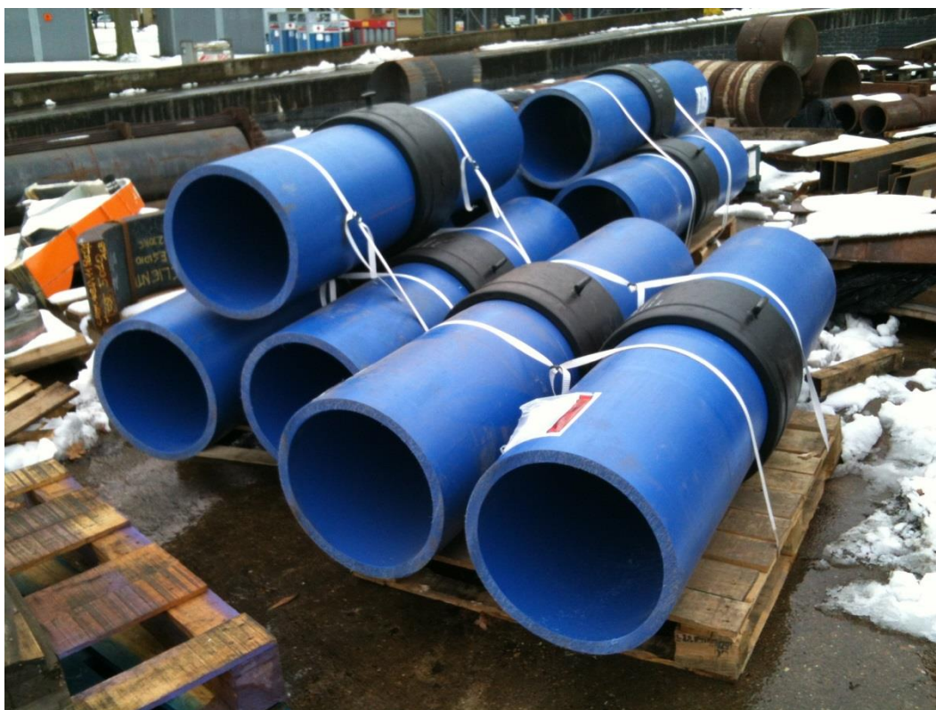
Figure 26 450mm electrofusion joints made in the project.
