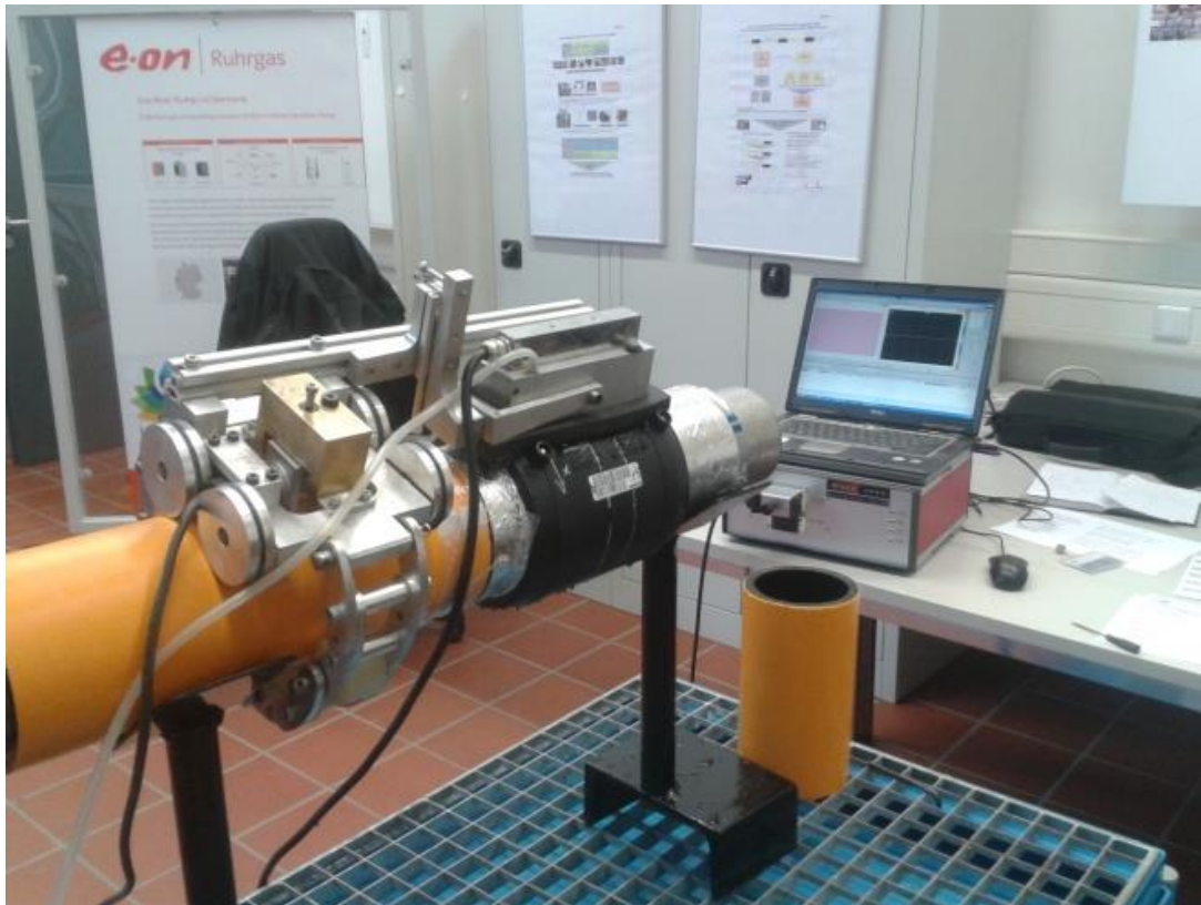
Figure 107 Inspection trials of EF welds at E.ON Ruhrgas.
