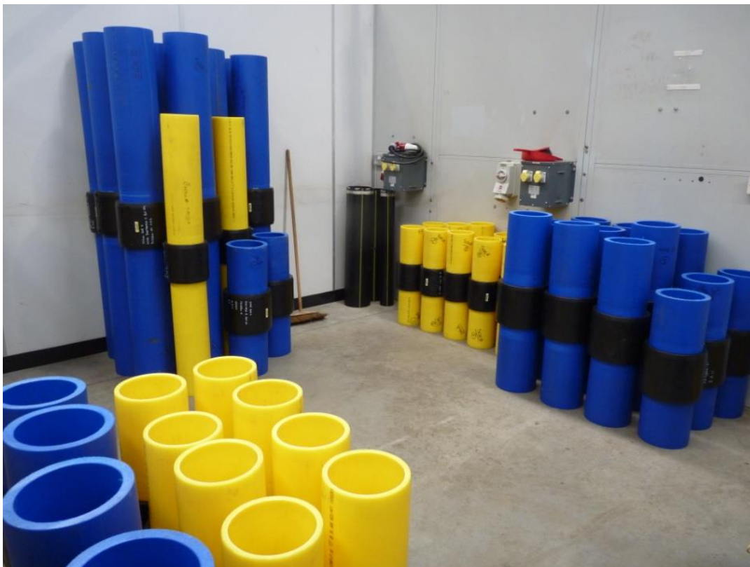
Figure 25 180mm and 225mm electrofusion joints made in the project.
