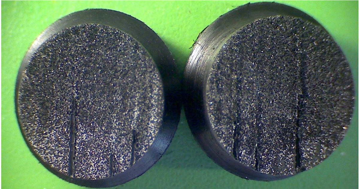
Figure 84 Typical appearance of an EF tensile creep rupture test specimens where rupture has occurred in the fusion plane due to sand contamination.
