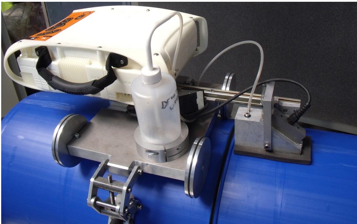
Figure 97 Carriage for inspecting large diameter pipes, with ultrasonic instrument and water reservoir attached.
