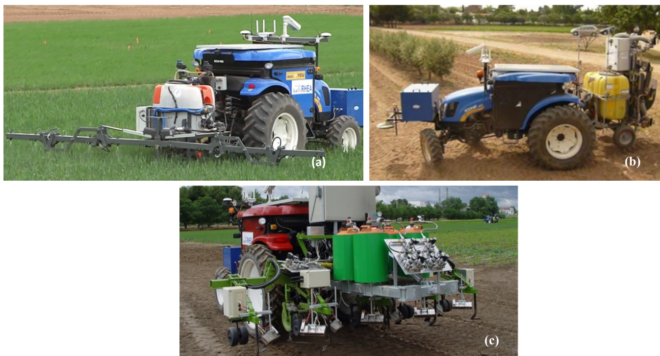
Fig. 4.1: (a) Patch sprayer; (b) Canopy sprayer and (c) Mechanical and thermal device
