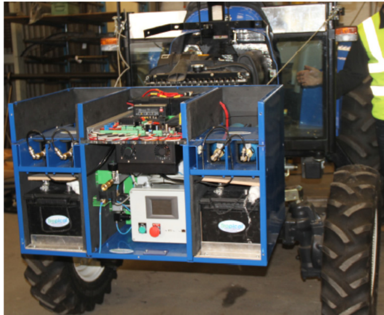
Fig. 5.5. Fuel cell system
