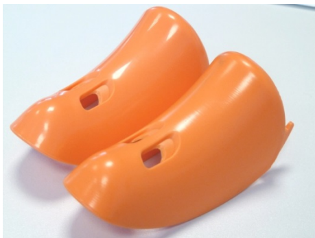
Figure WP7.3: Plastic Parts (front: manufactured from the laser polished mold, back: manufactured from the manually polished mold)
