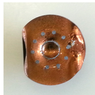
Fig. 29c: view through the membrane of the EAP prototype.
