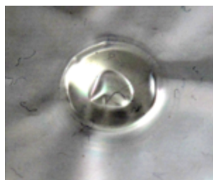
Fig. 16: Defect due to thermal shrinking at higher substrate temperature.
