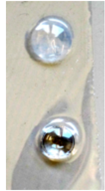
Fig. 22: Lenses ready for dicing by laser.
