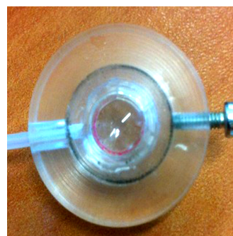
Fig. 30c: assembled lens + driver
