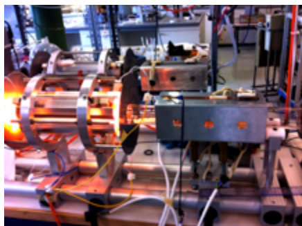
Fig. 8: LPCVD reactor for Parylene co-deposition containing two crucibles for two substances.
