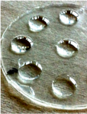
Fig. 19: Glass plate with RTV23 silicon moulds for trapping the liquid.
