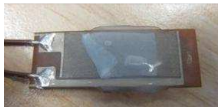
Figure 29 Encapsulated interdigitated electrode on flexible support.
