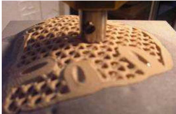
Fig. 4 PEEK scaffold testing: to validate the load-bearing resistance of the cranial implant. Ascamm (ES).
