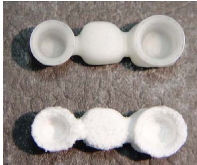
Fig. 9 Ceramic bridges produced by milling (top) in a commercial process, and laser melting (bottom) with the CustomIMD developed process. Bego (DE)
