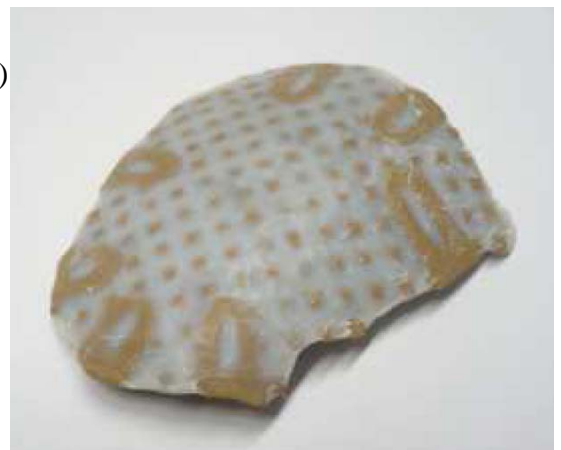
Fig. 6. Cranial implant design: a) Permanent PEEK scaffold guaranteeing the load bearing resistance. b) Implant ready for the surgery: PEEK scaffold + biodegradable osteoinductive composite. AZM (NL), EOS (DE), Suprapolix (NL), Xpand (NL), Ascamm (ES).
