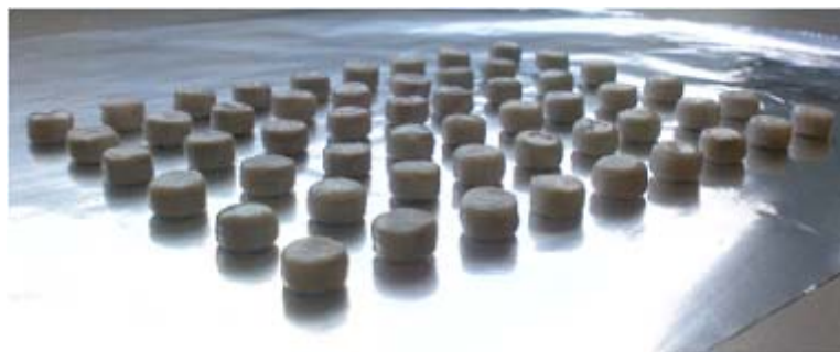
Fig. 5. Cylindrical PEEK meshes infiltrated with HA/SupraB-composite, used for animal testing of the cranial implant solution. AZM (NL), EOS (DE), Suprapolix (NL), Xpand (NL).
