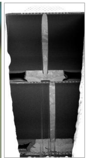
Figure 26. XSEM view showing 3 layer stacks.
