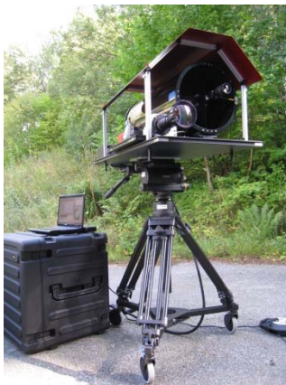
Figure 38. Left: sensor setup. The target substances were deployed on parts of a parked car at a distance of about 15m. Right: detection result. The system detected the DNT contamination (precursor of TNT) placed on the steering wheel. No false alarms for competing substances were generated.
