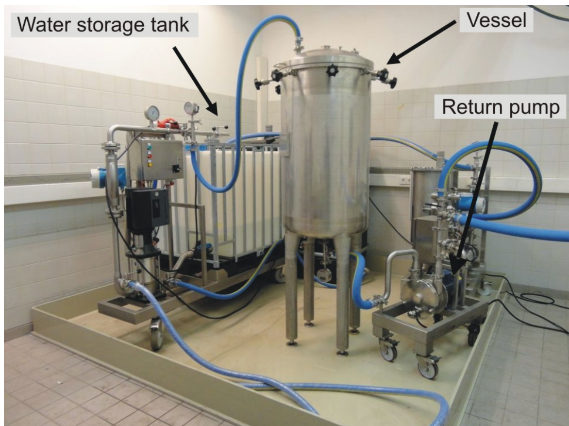
Figure 5: Picture of the experimental CIP plant for laboratory tests at TUW. The vessel in the centre of the picture is the object to be cleaned.
