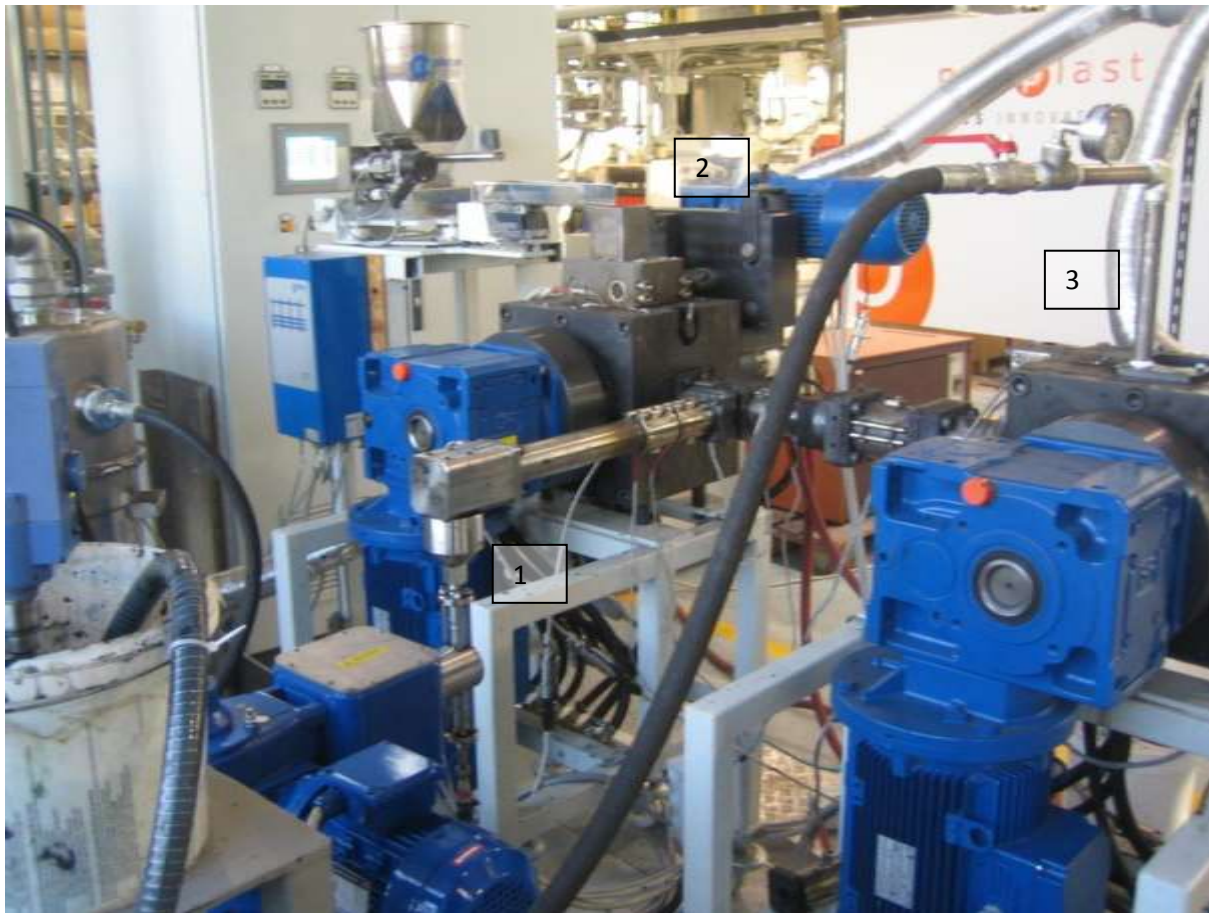
Figure 4.3.2: 1. Nexxus Melting NXBG200W80 ME, 2. Pumping group for the slurry, 3. Nexxus Degassing NXBG200W80 DE
