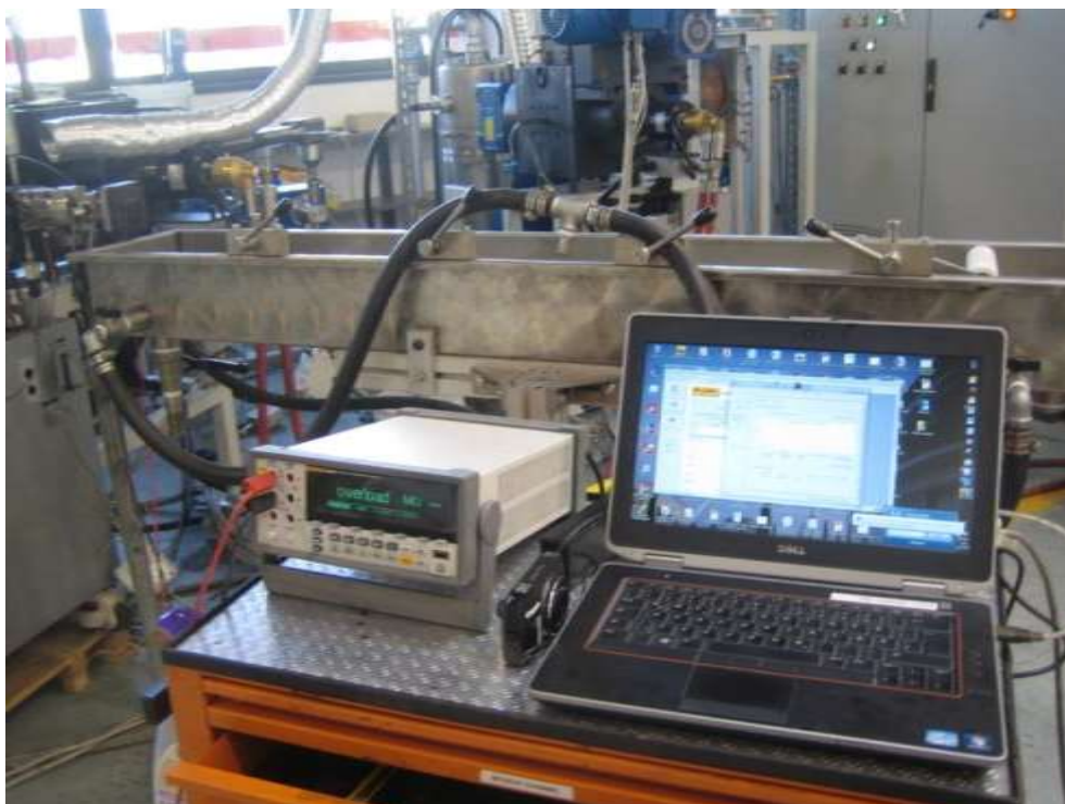
Figure 3.2.2.9: On line measurement of melt resistivity
