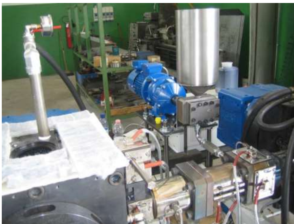
Figure 3.2.2.5. Early tests with waterborne CNT dispersion processed in Nexxus ((July 2013)
