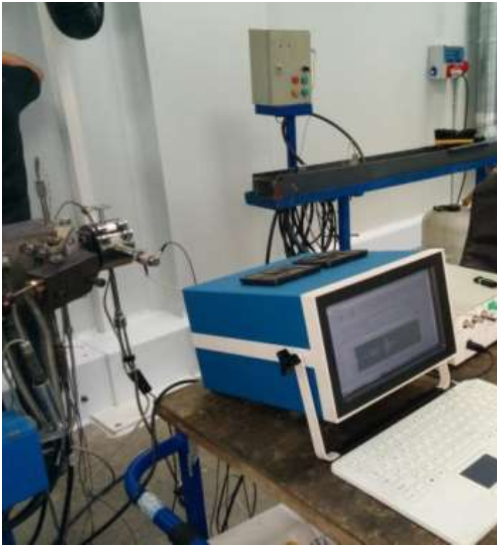
Figure 3.1.6.1: Global view of the ultrasonic measurement system
