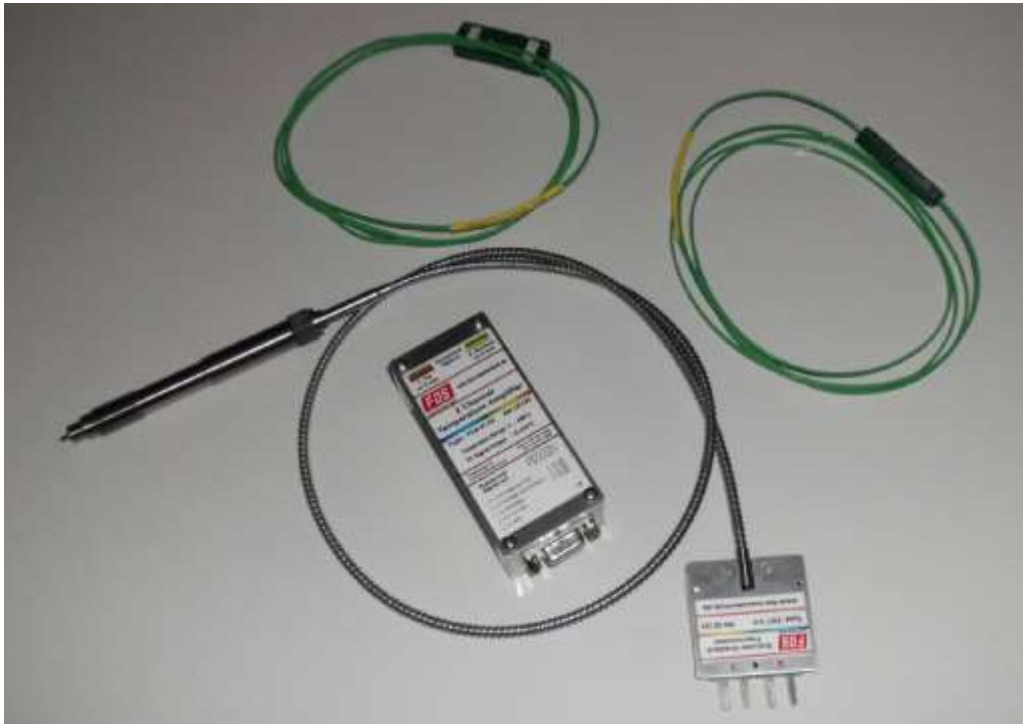
Figure 3.1.2.8: FOS multi point gradient thermometer measuring setup.
