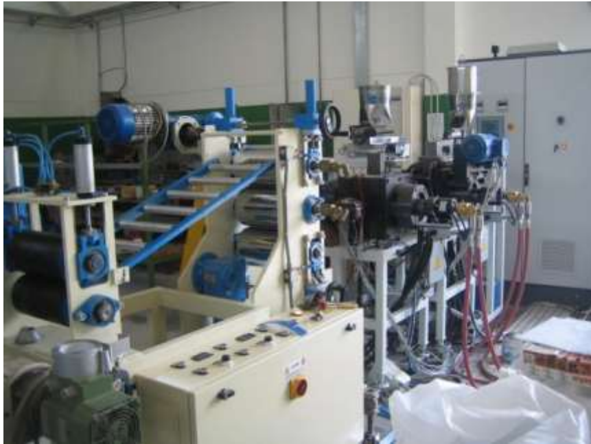
Figure 3.2.2.1: Nexxus Melting and Mixing in cascade
