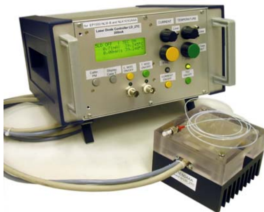
Figure 1.2 The 1389 nm repumper laser for the Yb clock
