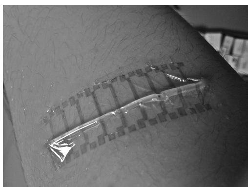
Fig 1: Conformal Organic Electrochemical Transistor with gel shown on a forearm.
