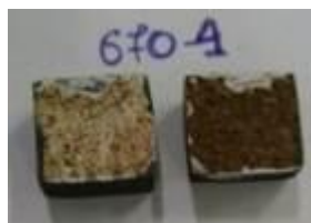
Figure 10: Norcoat fractured surface of \text{Al}_2\text{O}_3 -based adhesive (Ceramabond™ 670) C/C-SiC/Norcoat joint, mechanically tested at ambient conditions.
