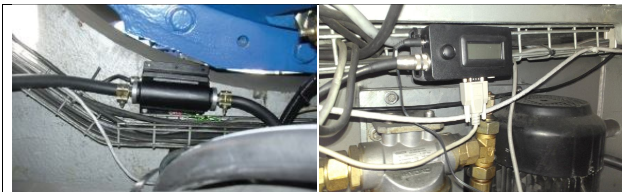
Figure 8 Oil sensor (left) and digital counter (right) installed on the NEG-MICON 750kW wind turbine at CRES's wind farm in Lavreotiki, Greece, the operational temperature range of the wear debris sensor is from -20°C to +65°C. The maximum permissible pressure of the oil is 10 bar
