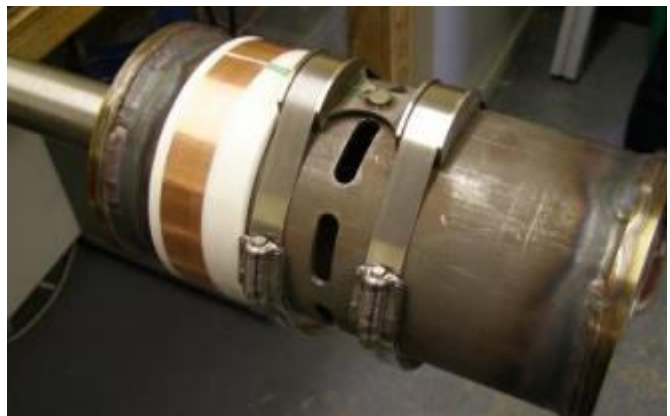
Figure 28 Two halves of the RF rotor coupler (left) and its installation on the test shaft (right)
