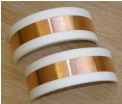
Figure 28 Two halves of the RF rotor coupler (left) and its installation on the test shaft (right)
