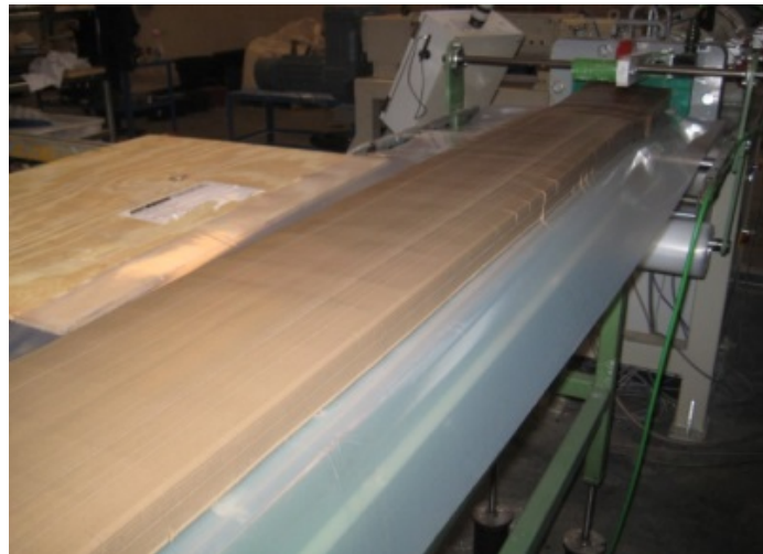
Figure 1.6. Extruded column of 3I binder
