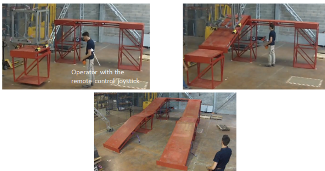
Footbridge assembly with generic platform
