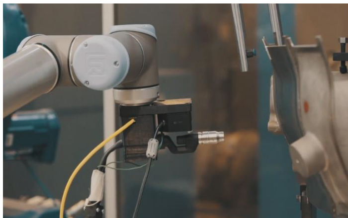
Figure 18: Automatic tack welding of the TRF at GKN
