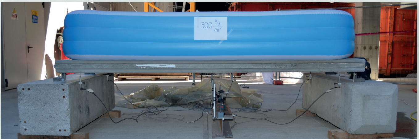
Figure 4: Experimental tests on simply supported real scale panel
