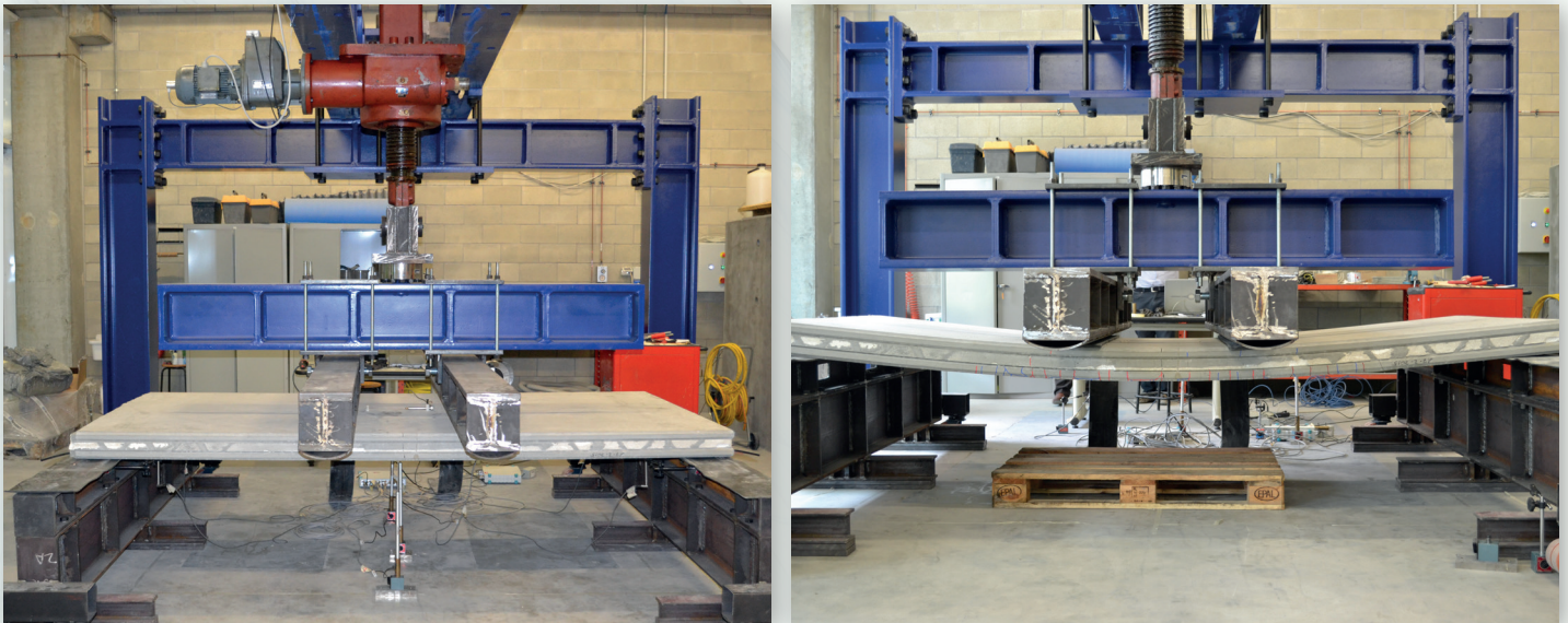
Figure 6: Displacement-controlled tests on simply supported real scale panel
