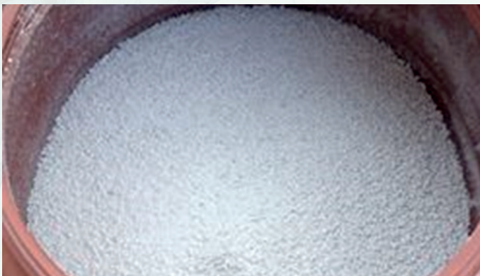
Loose hydrophobic perlite for insulation inside cavity wall
