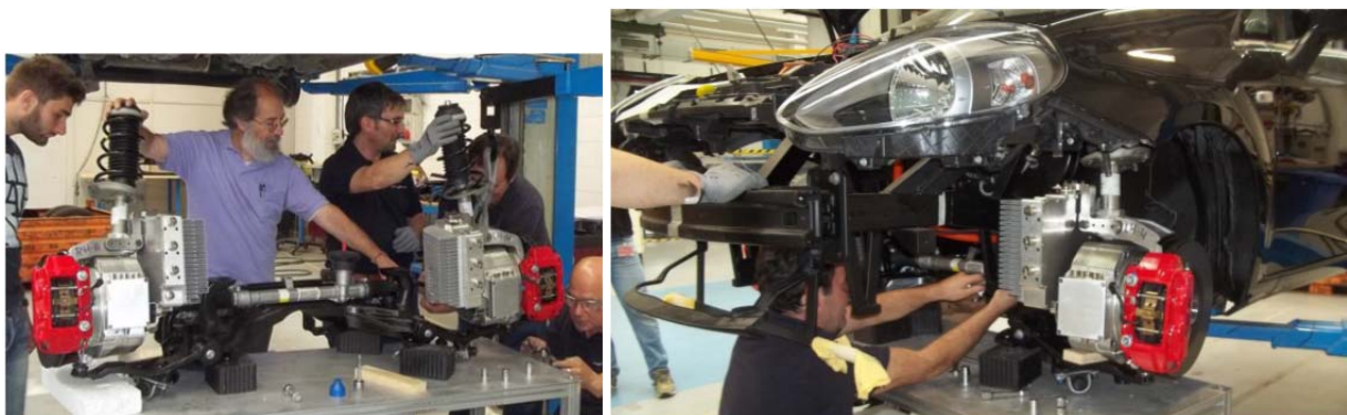
Figure 42: Final EUNICE in wheel system integration in donor car.
