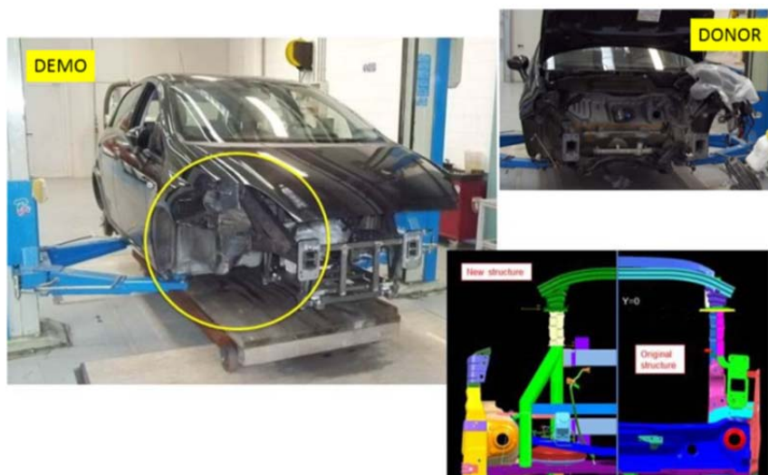
Figure 41: Final structural differences between donor and demo
