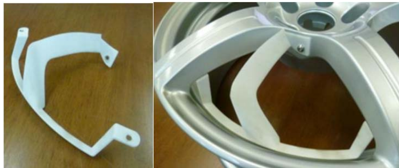
Figure 29: Turbine blade fixed on wheel
