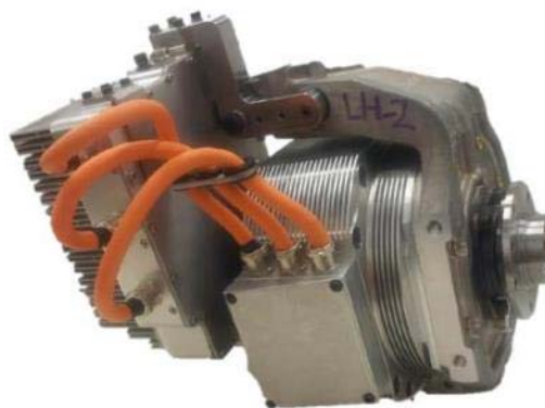
Figure 14: EUNICE electronic model and final prototype optimized for air cooling.
