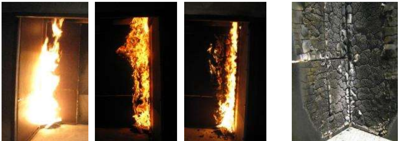
Figure 11. Uncoated furan-flax (cork core) sandwich panel (right: damaged surface after end of test)
