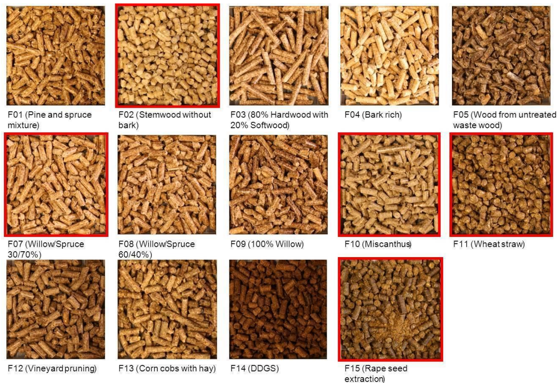
Figure 2: S&T results, Evaluation of laboratory tests - Fuels for laboratory tests (all pellets) and for boiler tests (pellets in red box) (source: TFZ)
