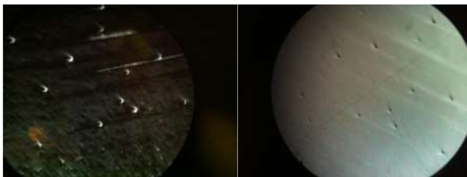
Figure 20: A sample with the presence of 4 \mu m silica beads aligned parallel and at 45° with respect to a set of crossed polarisers. The amplified signal exceeds 50 \mu m in size, which is on the limit of what can be appreciated with the naked eye
