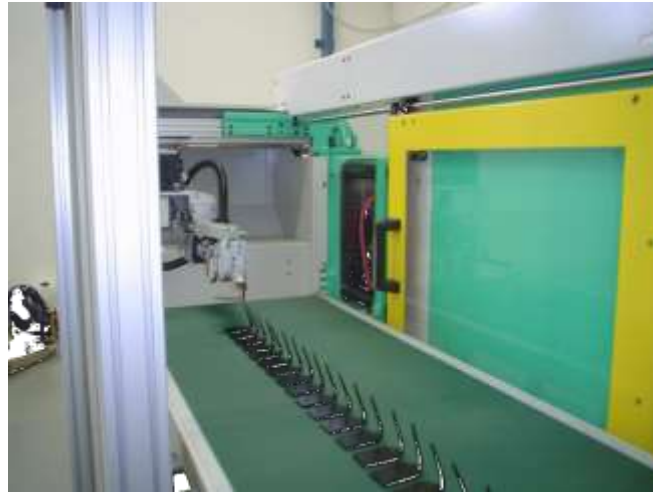
Figure 26: Automated production of injection moulded microfluidic cartridges
