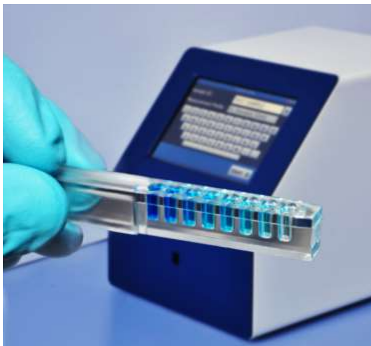
Figure 7: Picture of the core elements of the realized RaptaDiag EVA-Reader: EVA-Reader (background) and EVA-Chips (foreground)
