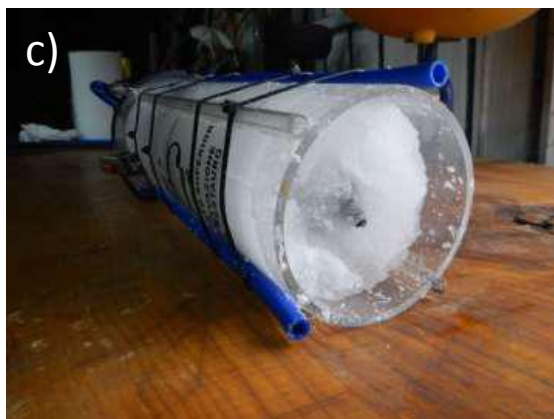
Figure 19. Use of the SAP system for consolidating sandy sediments in order to raise fragile artefacts
