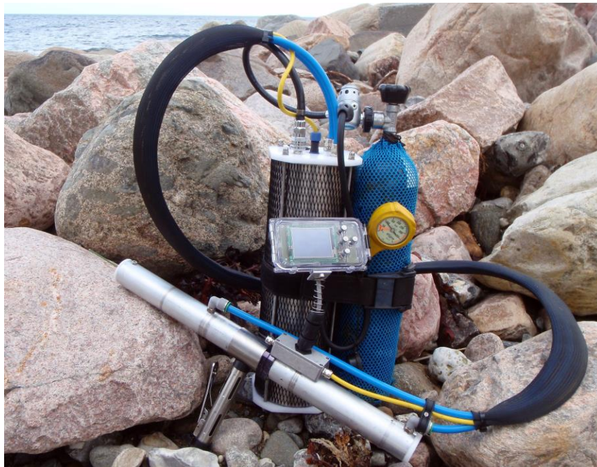
Figure 16: The diverheld underwater wood tester (WP4UW)
