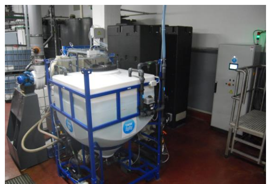
Figure 6: The 2 MHD evaporation units and its control system implemented in the ECOWAMA pilot plant
