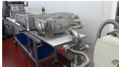
(c) vacuum test after welding
