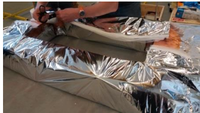
(b) MLI blankets installation
