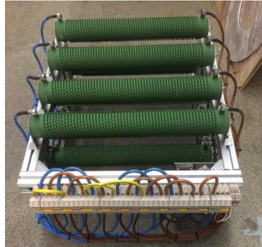
Figure 21. (Left) Quench protection scheme (Right) Stationary resistors bank
