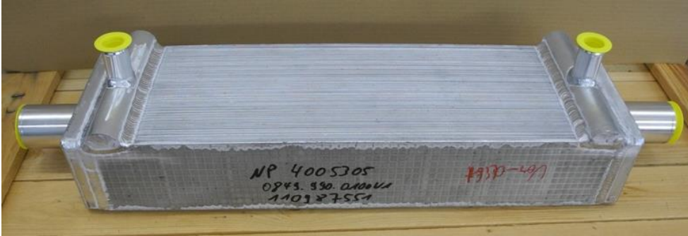
Figure 23: Photo of condenser
