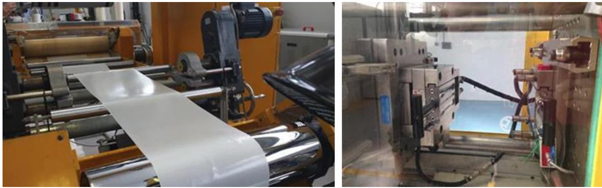
Figure 53: Cast-sheet extrusion and test bar injection of additived InnoREX PLA compound
