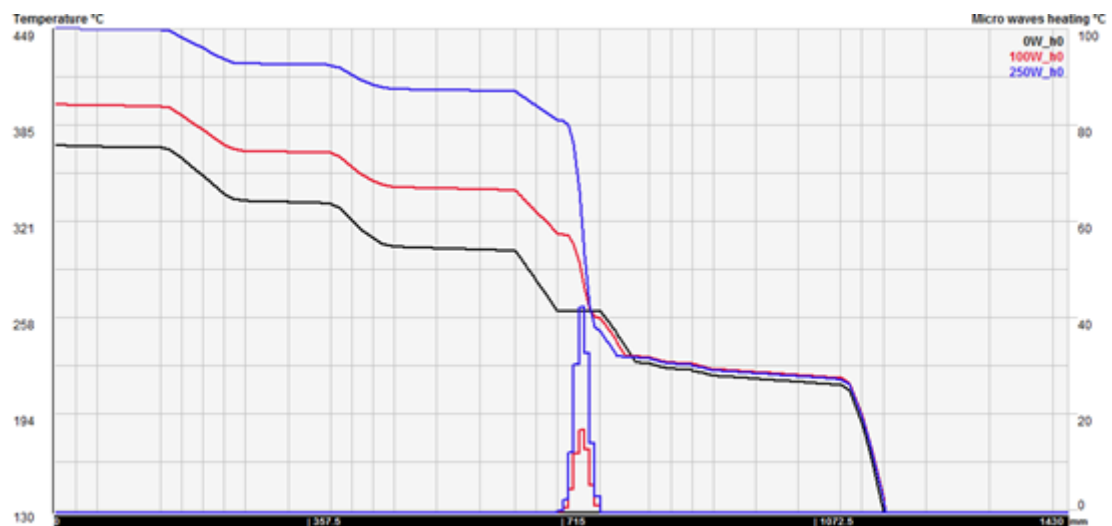
Figure 45: Effect of level of microwave power on temperature
