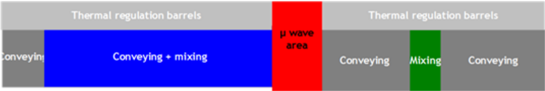
Figure 40: Screw profile with microwave device
