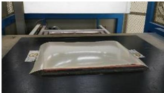
Positioning the sheet in the forming area
