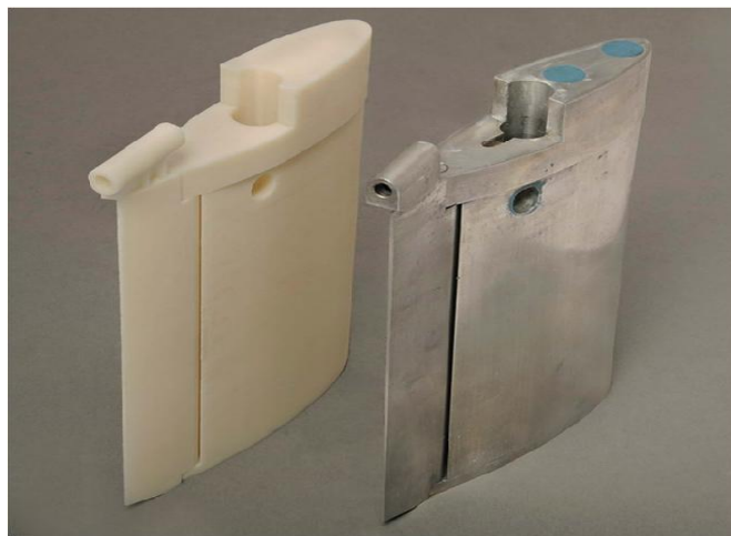
Fig. 10: Flap rudder made by RPT (left) and milled aluminium (right).
